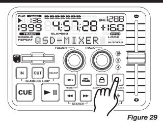
**Using the Pitch Slider Percentage Selector** (28): You may choose a pitch operating range at any time. To change the operating range be sure the pitch function is turned on, see figure 27. The pitch percentage can be changed between +/-4%, +/-8%, or +/-16%. 4% will allow the least amount of pitch manipulation and 16% will allow the most amount of pitch manipulation. To adjust the different values, hold the % BUTTON (28) until your desired value is reached.
